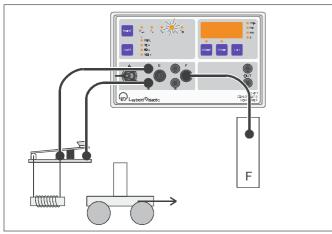
Measuring the time from the start of the motion (interruption of a circuit involving the holding magnet) until the trolley reaches the light barrier.
