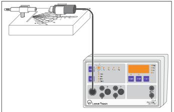
The pulses are triggered by radioactive radiation in an endwindow counter. An arbitrary gate time can be selected.
