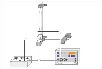
Generating standing waves on a rubber string (or on a helical spring) with a motor and a tacho-generator, which is driven by the function generator.
