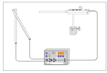
Measuring the propagation time between the sound generation (by slamming together the two stand rods) and the sound detection by the multi-purpose microphone.
