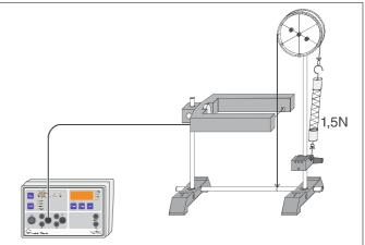
Counting the number n = 2 f of light barrier interruptions per second caused by the oscillating string.
