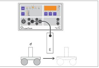
Measuring the interruption time of the light barrier E and calculating the average velocity during the interruption from the width of the interrupter flag according to v=d/t.
