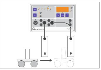
Measuring the time interval beween the interruptions of the light barrier E and the light barrier F.
