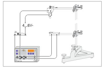
Measuring the time from the start of the motion (interruption of a circuit involving the holding magnet) until a contact is made (the experiment body reaches the contact plate).
