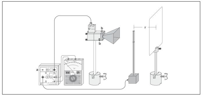
Fig. 3 Experimental setup for determining the wavelength on standing microwaves
