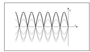
Fig. 1 Standing wave ratio (---) and oscillatory states (- -) of the electric field of a standing microwave
