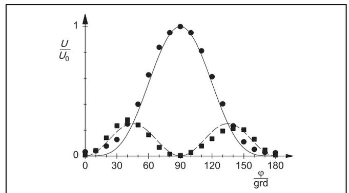
Fig. 7 Normalized received signal behind the polarization grating with the E-field probe being aligned vertically
