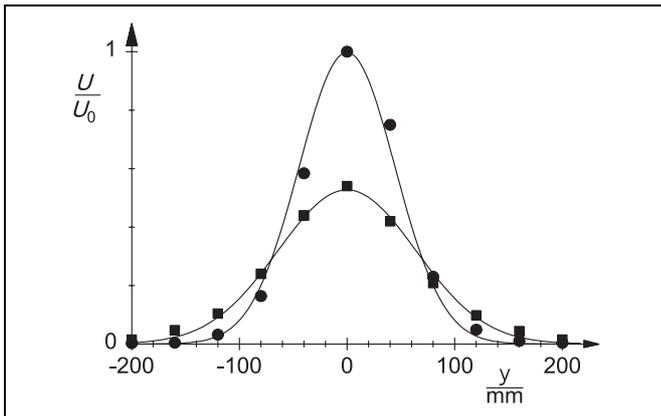
Fig. 5 Transverse distribution of the normalized received signal in front of the horn antenna (● :  $x_0 = 100$  mm, ■ :  $x_0 = 200$  mm)
