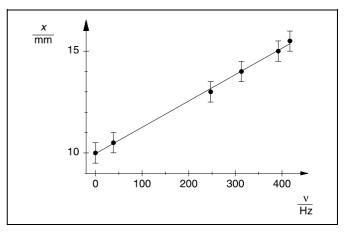
Fig. 4: Position x of image S" on the glass scale as a function of the motor frequency  $\nu$ .
