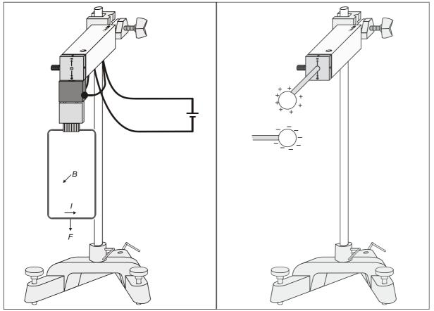
The force sensor is fixed via a short stand rod and used in a way that forces can be easily measured in two directions (in contrast to electronic balances).
