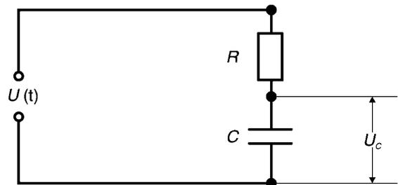
In the experiment, the square-wave voltage  $U(t)$  and the voltage  $U_C$  at the capacitor  $C$  are displayed on the oscilloscope. The half-time  $T_{1/2}$  is determined from the time base sweep.
