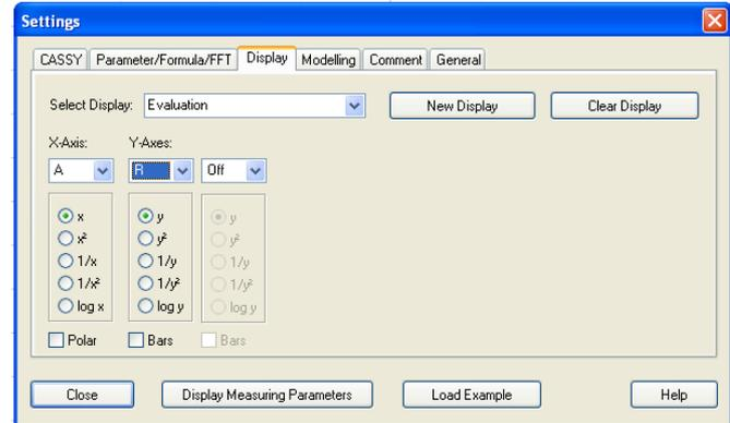
If you perform a fit of a straight line trough origin the drag and drop capability of the software allows you to shift the result of the fit (i.e. the value of the determined resistance) into the table of the new defined Display "Evaluation".
