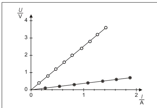
Fig. 4: Relation between the voltage  $U$  and the current  $I$  for constantan wire (○) and brass wire (⊙) with equal cross-sectional area and equal length
