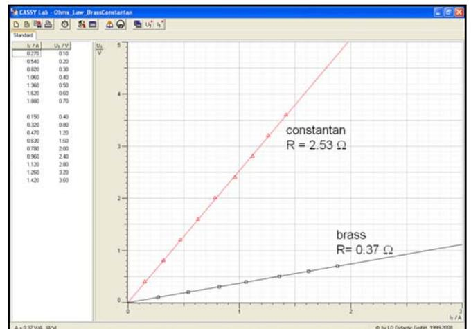
The measurement series on brass 0.5 mm dia. in steps of 0.1 V and the measurement series on constantan 0.5 mm dia can also be performed in a similar manner. The measuring results with CASSY are shown in the following picture:
