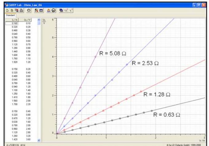
The measurement series for constantan wires 0.7 mm dia. (total length  $\ell = 1$  m and  $\ell = 2$  m) can be performed in similar manner. The measuring results with CASSY are shown in the following picture:
