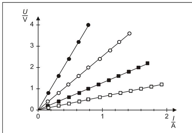
Fig. 2: Relation between the voltage  $U$  and the current  $I$  for constantan wires with the cross-sectional areas  $A = 0.1 \text{ mm}^2$  (●),  $0.2 \text{ mm}^2$  (○),  $0.4 \text{ mm}^2$  (■) and  $0.8 \text{ mm}^2$  (□)
